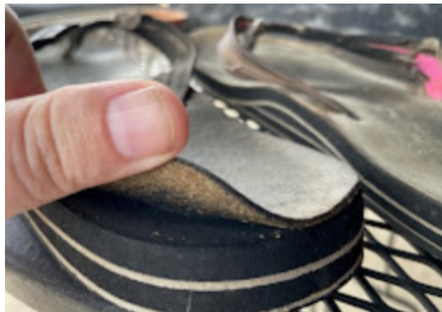
Figure 2 Delamination of Mr. Sher's sandal.
